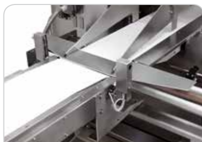
Belt type in-feed conveyor
