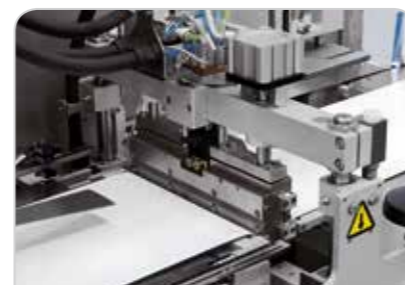
Cross sealing head designed to guarantee high quality hermetic seals
